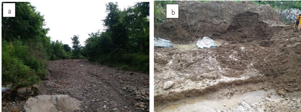
Photograph 0-3: a. Debris flow at Chanabari Khola, and b. Silty clay soil at Solighoptegaun
