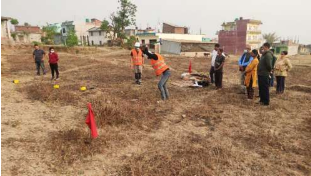
Photograph 0-24 Geophysicist, Geo Engineering Consult Pvt. Ltd. demonstrating the active seismological survey technique to the municipal team.
