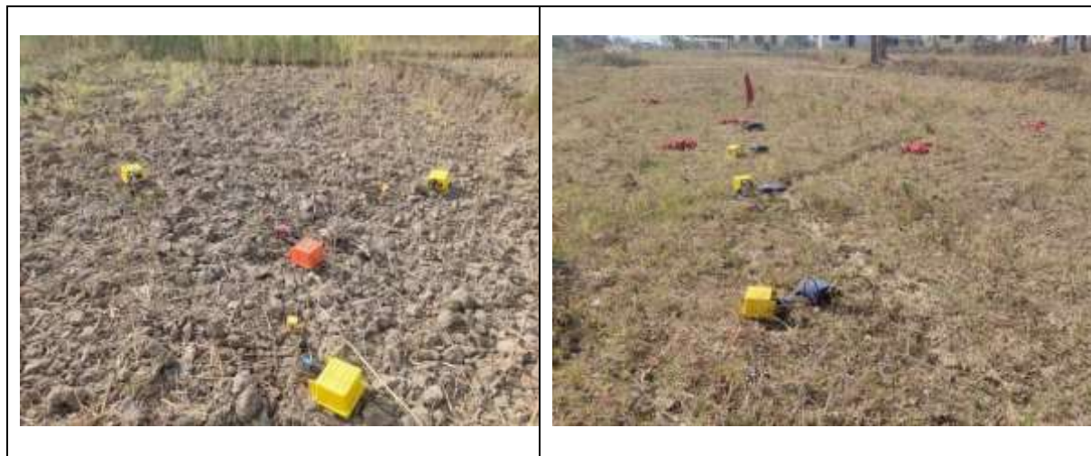
Figure 0:18 (a) Tripartite array (b) Line array for ambient noise array measurement.
